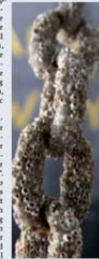
FOULED: Ships are more prone to barnacle build-up in tropical waters, as on this anchor chain. PHOTO: SCANPIX
