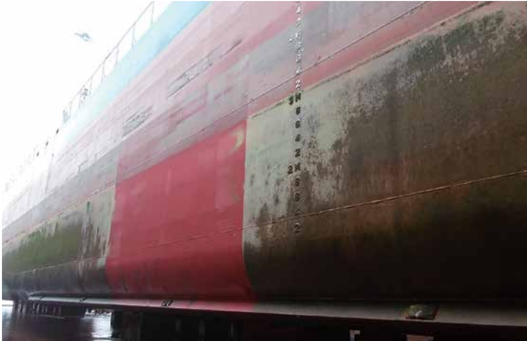
Chugoku Marine Paint test patch of antifouling coating using Selektope® on Japanese coastal vessel after two years
