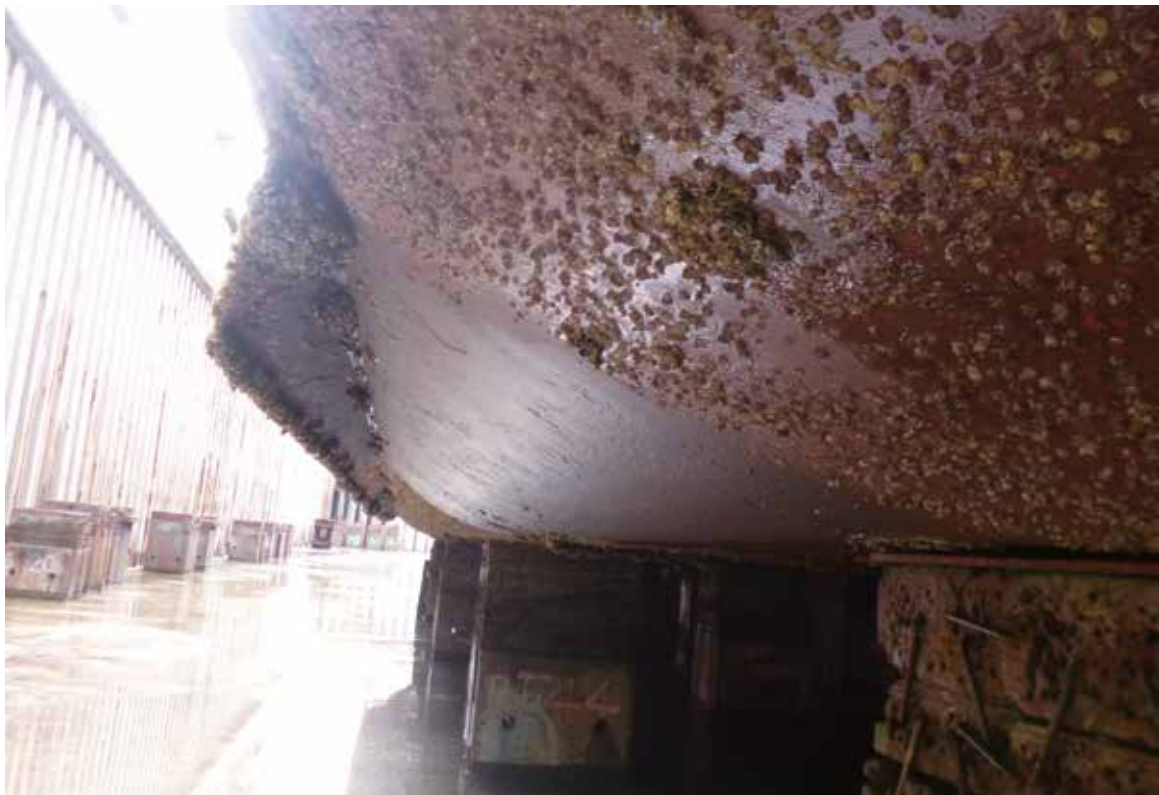
Chugoku Marine Paint hull bottom test patch of antifouling coating using Selektope® after one year trials on low activity coastal vessel in Tokyo Bay (high fouling area)
