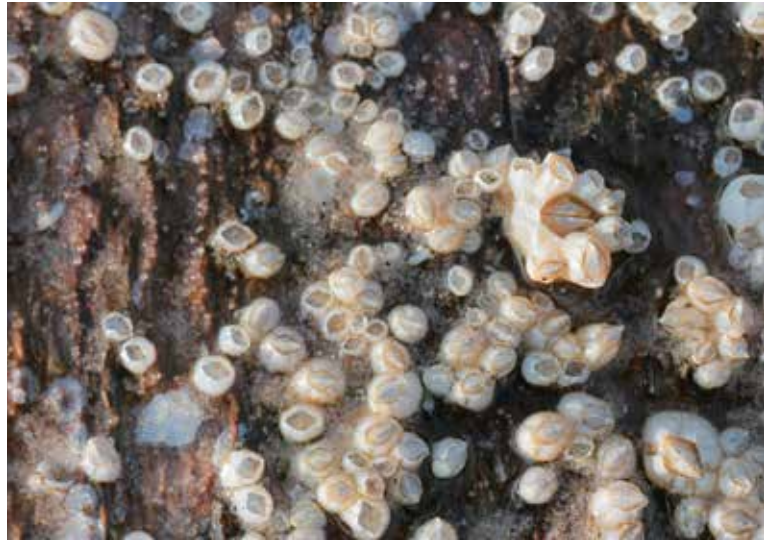
Barnacle built up on test patch after seven months in static condition on west coast of Sweden using antifouling without Selektope®
