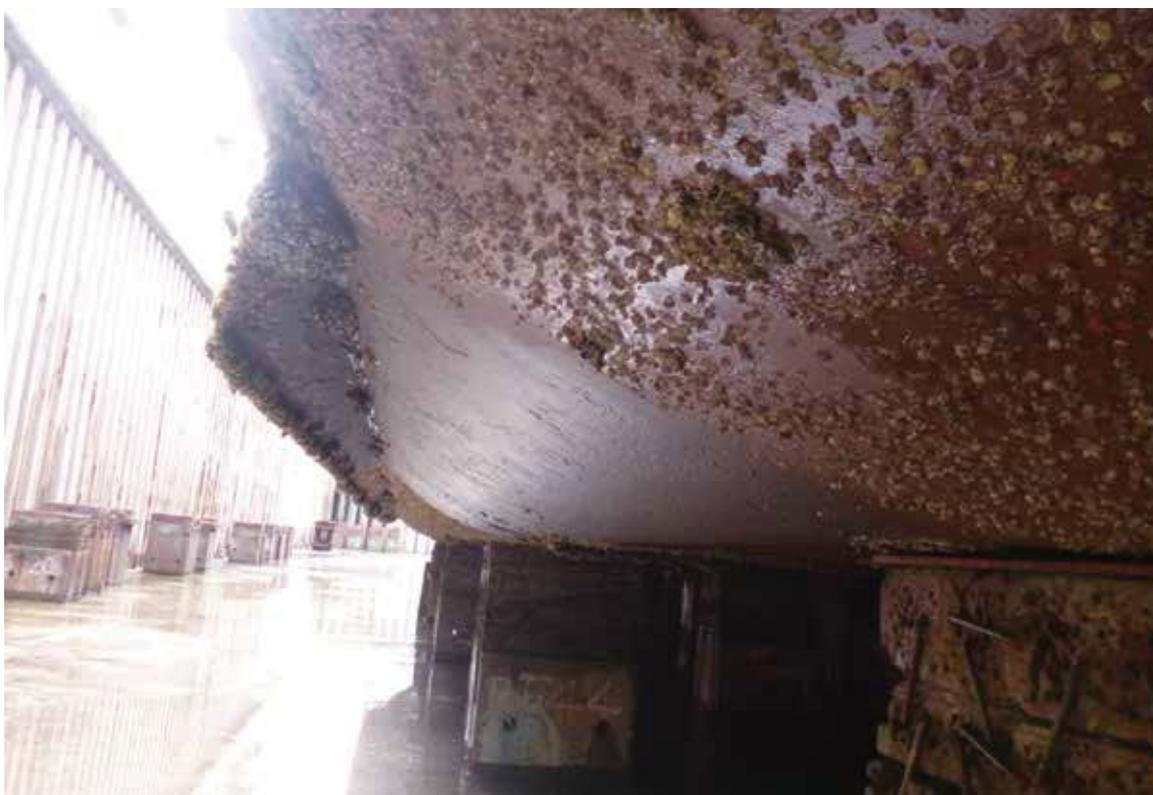
Chugoku Marine Paint hull bottom test patch of antifouling coating using Selektope® after one year trials on low activity coastal vessel in Tokyo Bay (high fouling area)
