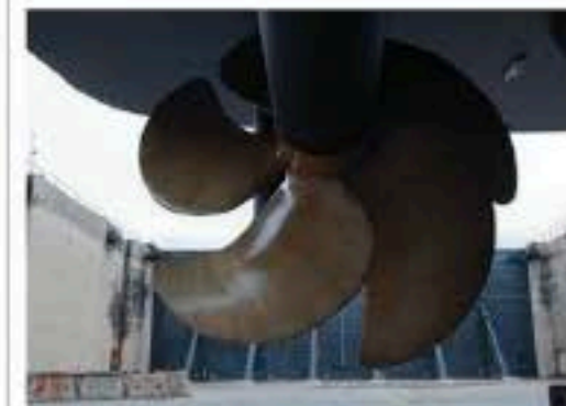
A wide range of foul release coatings has been developed for propellers, such as Ecoshield from Subsea Industries which has been designed to withstand cavitation damage
