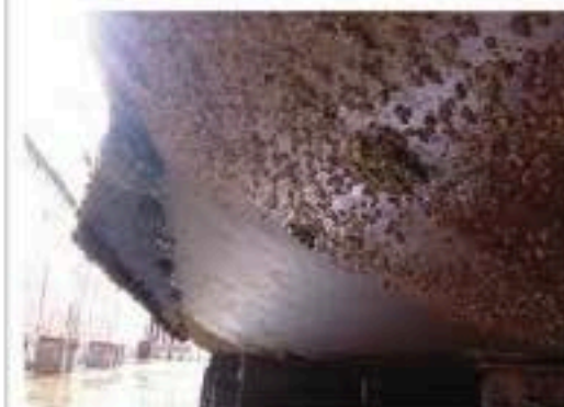
The results from a two-year test patch trial of Selektepe on the tanker Calypso . Independent verification suggests steady performance against variables
