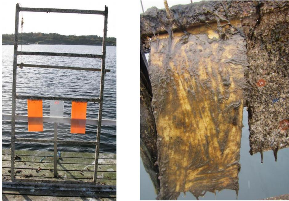
Fig 15. Three-panel polyurethane test conducted with only one formulation containing 0.37% Selektope® versus a reference panel with 0% Selektope® - October 2015 - November 2017
