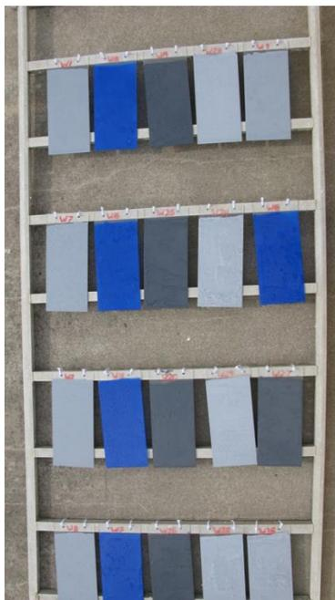
Fig. 16. Reference silicon epoxy-coated test panels submerged in April 2016 off the west coast of Sweden.
