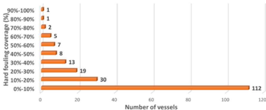
On 44% of vessels surveyed, over 10% of the underwater hull surface was significantly covered with hard fouling. On many vessels, fouling levels were even worse; approximately 15% of vessels had between 10-20% of hard fouling coverage on the hull, 10% of vessels had 20-30% of hard fouling coverage and the remaining 10% of vessels had be-
