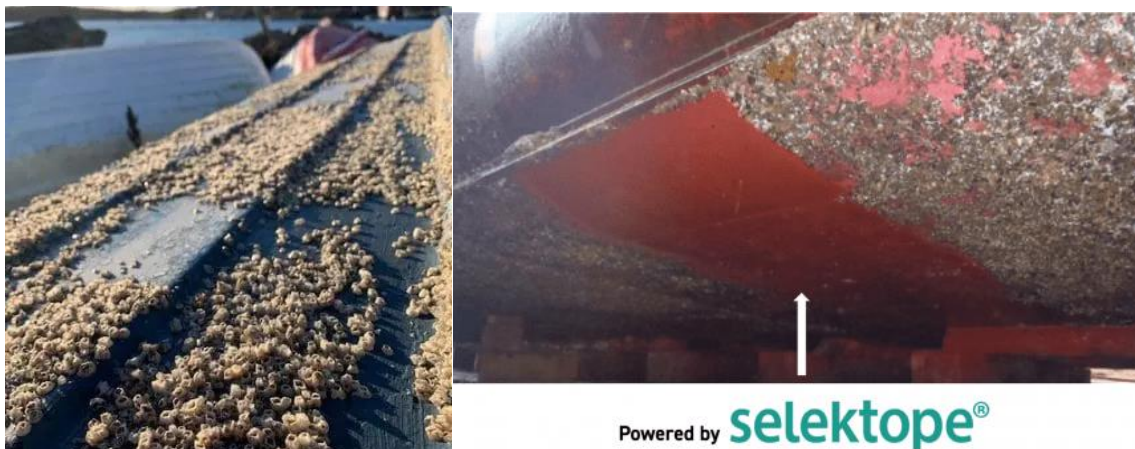
Left: Ship hull covered with hard fouling. Right: Comparison of ship hull sections treated with and without Selektope®.
