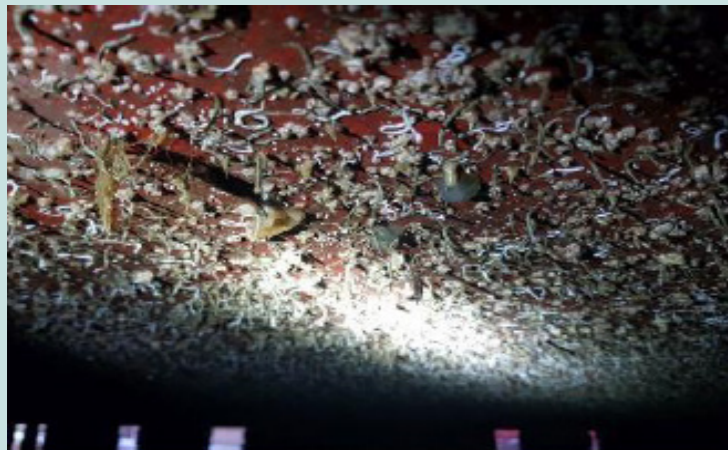
Vertical sides of the underwater hull area of a LNG carrier with an FRC coating. In service period: Unknown.
